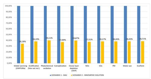
Comparison between the results of the Scenario 1- Yacht with traditional HVAC system (BAU) and Scenario 2- Yacht with innovative HVAC system (Innovative Solution). The results are expressed in percentage.
